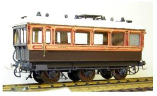
The third item is a chassis for a LSWR 6-wheel 33ft Brake composite saloon. Originally built in 1896 it was converted with the addition of guards compartment (replacing the luggage compartment) in 1912. I have yet to make a start on the body. The chassis is of the Clemison type where the centre axle can move from side to side with the curves.
