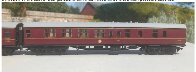
(Above) The almost complete Corridor Brake Second. Roof still to be painted, weathered and fixed in place. The interior wood panel colour comes through in this shot.
